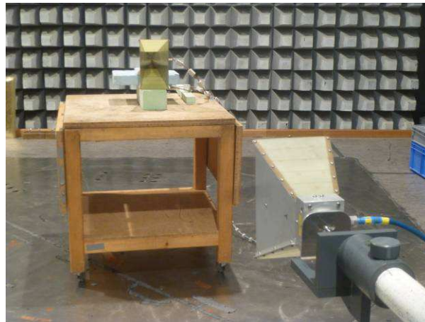
Figure 1-3: Reference measurement, 1 – 6 GHz
